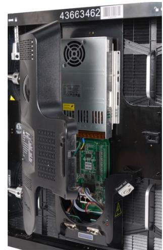
AV6XS: Quick-Release Power Supply with 4X Receiver Card Modules. Modules are secured with magnets and set screws.
