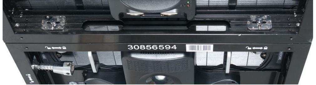
2. Push locking vertical connectors up through their corresponding slotted vertical tab-keyed connector sockets
