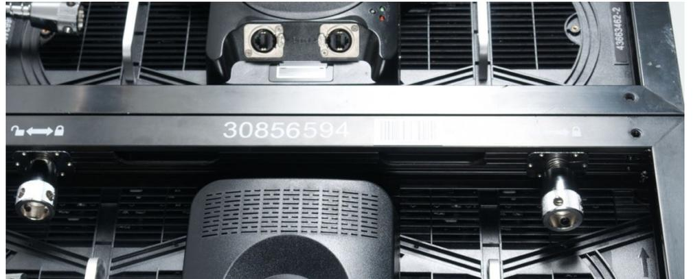
3. Compress spring of vertical panel connector and pass locking-tab through tab-keyed connector socket
