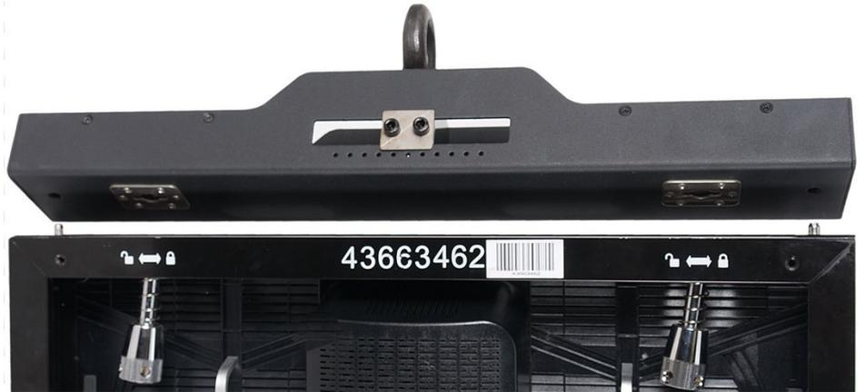
2. Push locking vertical connectors up through their corresponding slotted vertical tab-keyed connector sockets in the AV6RB2 Rigging Bar, and compress spring of vertical panel connectors and passing their locking-tab through tab-keyed connector socket, and turn 90° to lock
